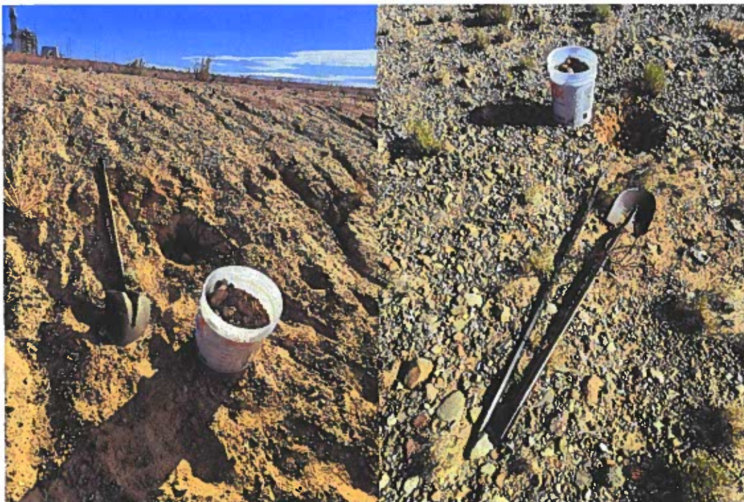
Figure 17. In-bank Fine and Gravel cover material in borrow pit.
