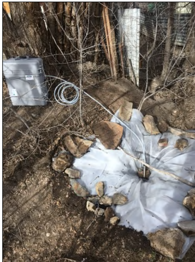
Water Quality Monitoring Site DP2 , second discharge point representing cumulative stormwater runoff within APE before discharging into the unnamed ephemeral stream
