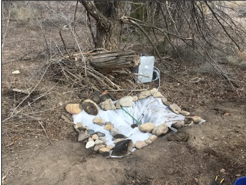
Water Quality Monitoring Site DP1 , first discharge point representing cumulative storm runoff within APE before discharging into the unnamed ephemeral stream
