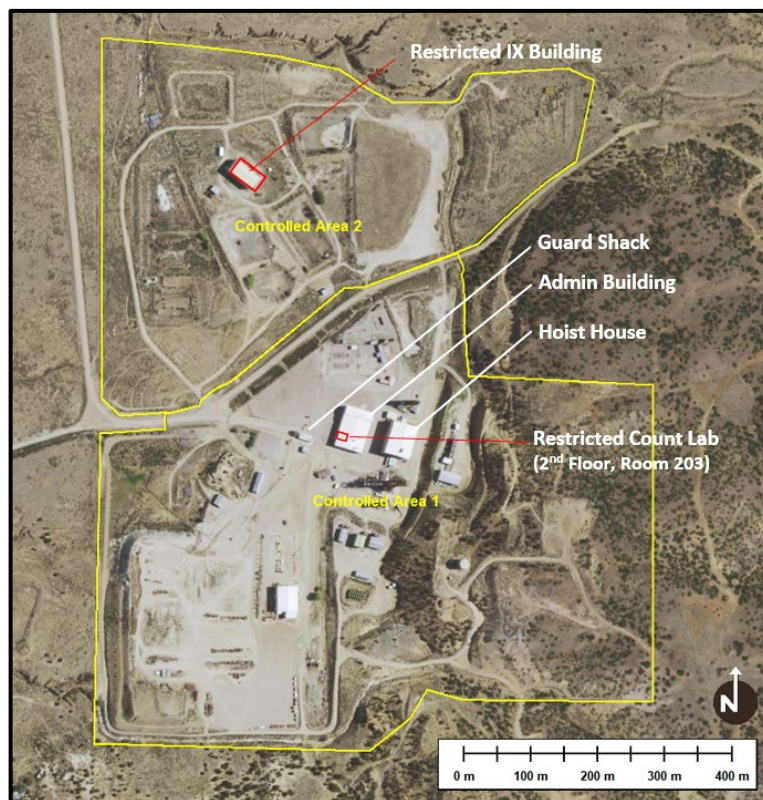
Figure 3: Site layout for Controlled and Restricted Areas.
