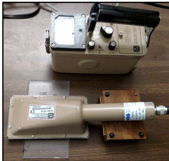
Figure 3-1: Example fixed-geometry measurement jig using a Ludlum 43-93 survey probe (to count swipe samples, determine instrument efficiency, and to perform daily QC function checks).
