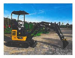
John Deere 17G Mini Trackhoe with a 15" wide bucket. Model unit weight is 3,800lbs. Rubber track system with a blade. This unit is purchased near new condition with zero hydraulic leaks, no oil or fuel leaks, all equipment has been tested and reviewed by a local dealership in Las Cruces, NM. Unit will be used on-site to facilitate the digging of material through the placer. Unit will be only stored on-site when operations are in an active phase. When work is on hold or the
