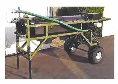
Custom Trommel/Highbanker for processing placer material. This trommel/highbanker is 10' long, 5ft wide, and 4' tall. The sluice box that attaches to it for the concentration of material is 10' long. This unit allows for an average maximum of 7 tons of raw unclassified material per hour, equating to 3 to 5 cubic yards per hour of material processing. This unit is portable via
