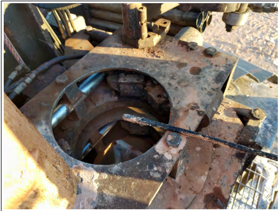
4. Water level in dry borehole measured after borehole open for one hour
