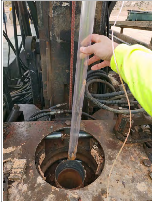
3. Bailer test for significant water after borehole open for 15 hours (overnight)
