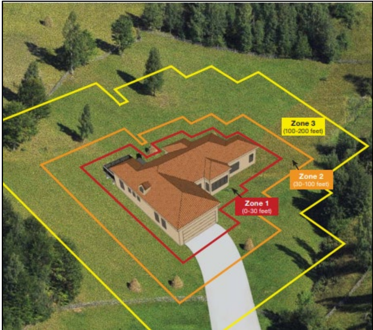
Figure K.1. Defensible space zones providing clearance between a structure and adjacent woodland or forest fuels.
