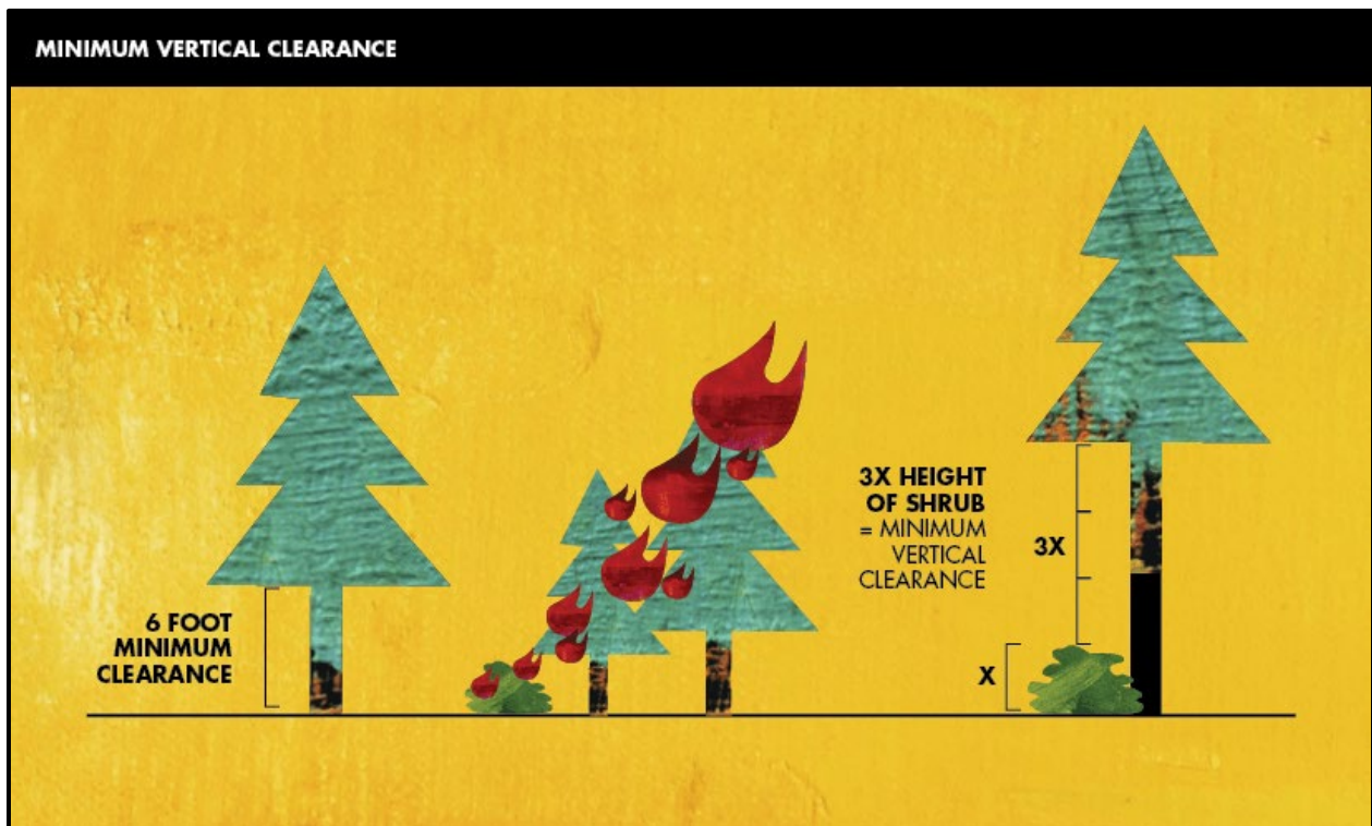
Figure K.3. Minimum vertical clearance.
